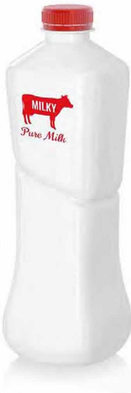
The original pennaholt enabled typical 8%  $TiO_2$  content in a PET bottle for long life white milk to be cut to below 4% in monolayer PET bottles and below 2% in multilayer packages. This helped to improve white opaque PET’s compatibility with the non-clear recycled PET stream, where high content of  $TiO_2$  had previously been identified as hindering both the recycling process and the manufacture of end-products using non-clear rPET content.
